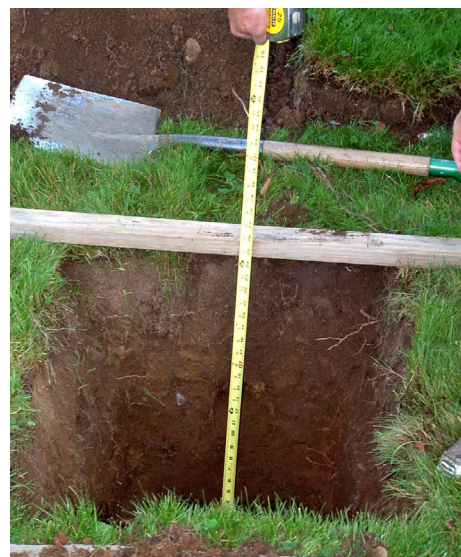
A pit test to calculate soil drainage rates is a critical first step. Photo: Erica Guttman
