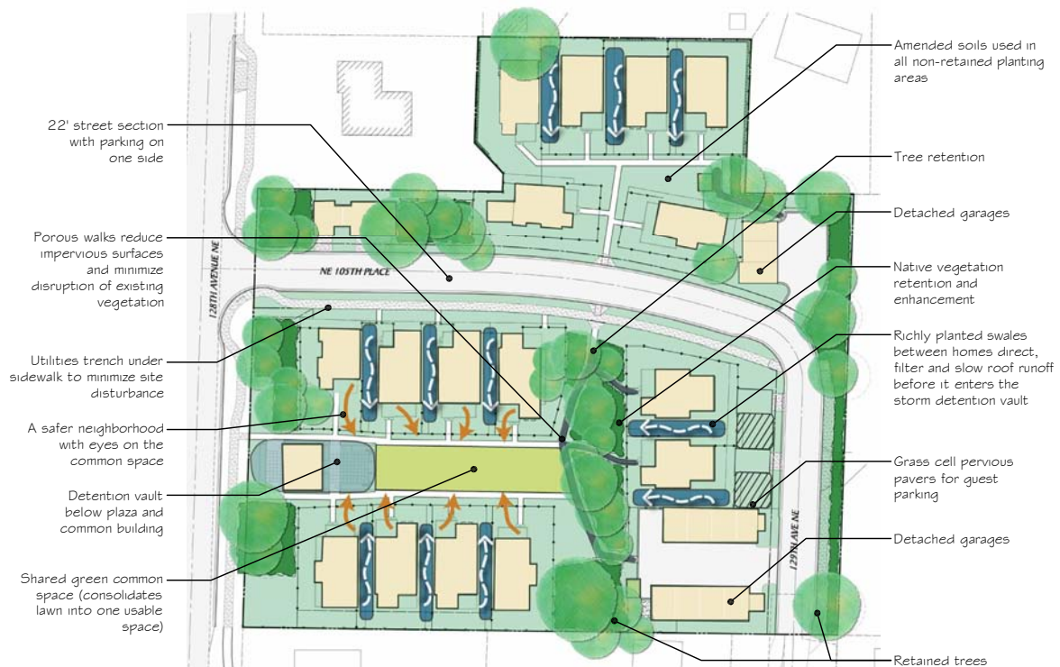
DANIELSON GROVE Sustainable Components Plan Graphic by Triad Associates for The Cottage Company
