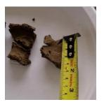
**5 – Measure the ribbon length**. By measuring the ribbon length, record this.
