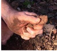
**8 – Determine the soil type by comparing it to the Matrix Key**. Check the combination of soil ribbon length and texture against our Soil Texture Matrix. By using the rows as classified by ribbon length, and the columns classified by texture, you can determine the soil type. This is comparable to the NRCS soil texture pyramid.
