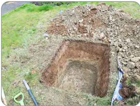
Make sure your test hole is three feet deep. Soil textures can vary with depth.
