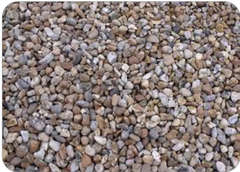
Washed drain rock is the best material for underground infiltration systems.
